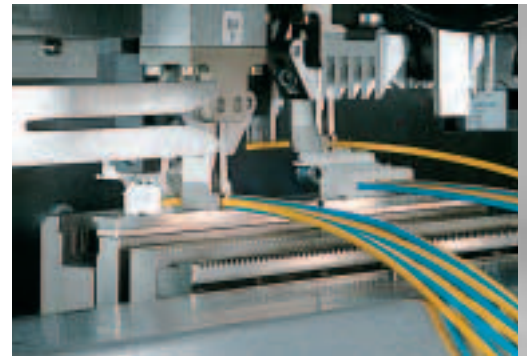
Insertion of IDC connectors
