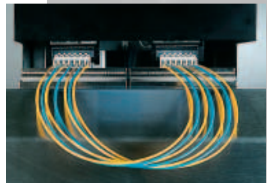
Optical test of insertion depth
